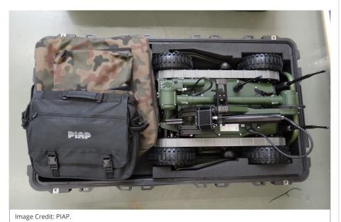
The operator, by the means of utilizing the robot, would be able to search the means of transport for presence of dangerous objects, or inspect ditches and tunnels under the roads. The observation capabilities were to be offered by high resolution cameras with IR illumination system, daytime/night camera and a thermal vision camera.
