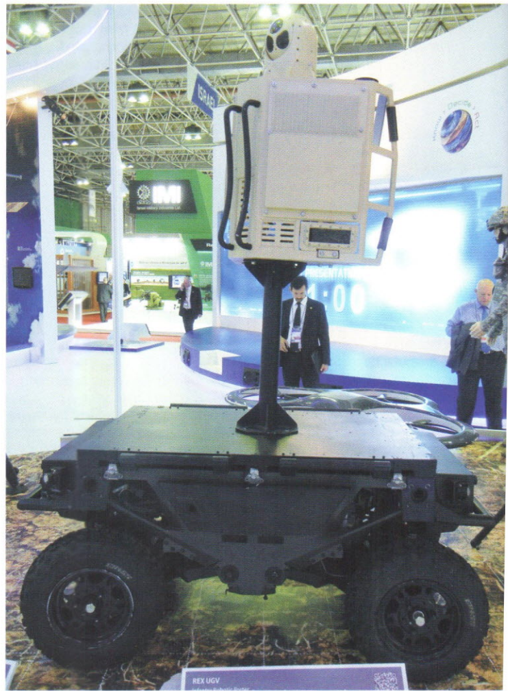
Israel Aerospace Industries' (IAI) REX is meant to carry any payload of up to 200kg, including munitions, weapons, and logistics, to increase mobility of combat troops, particularly Special Forces. The vehicle, with an 11hp engine, could be programmed to maintain the pace of soldiers.
