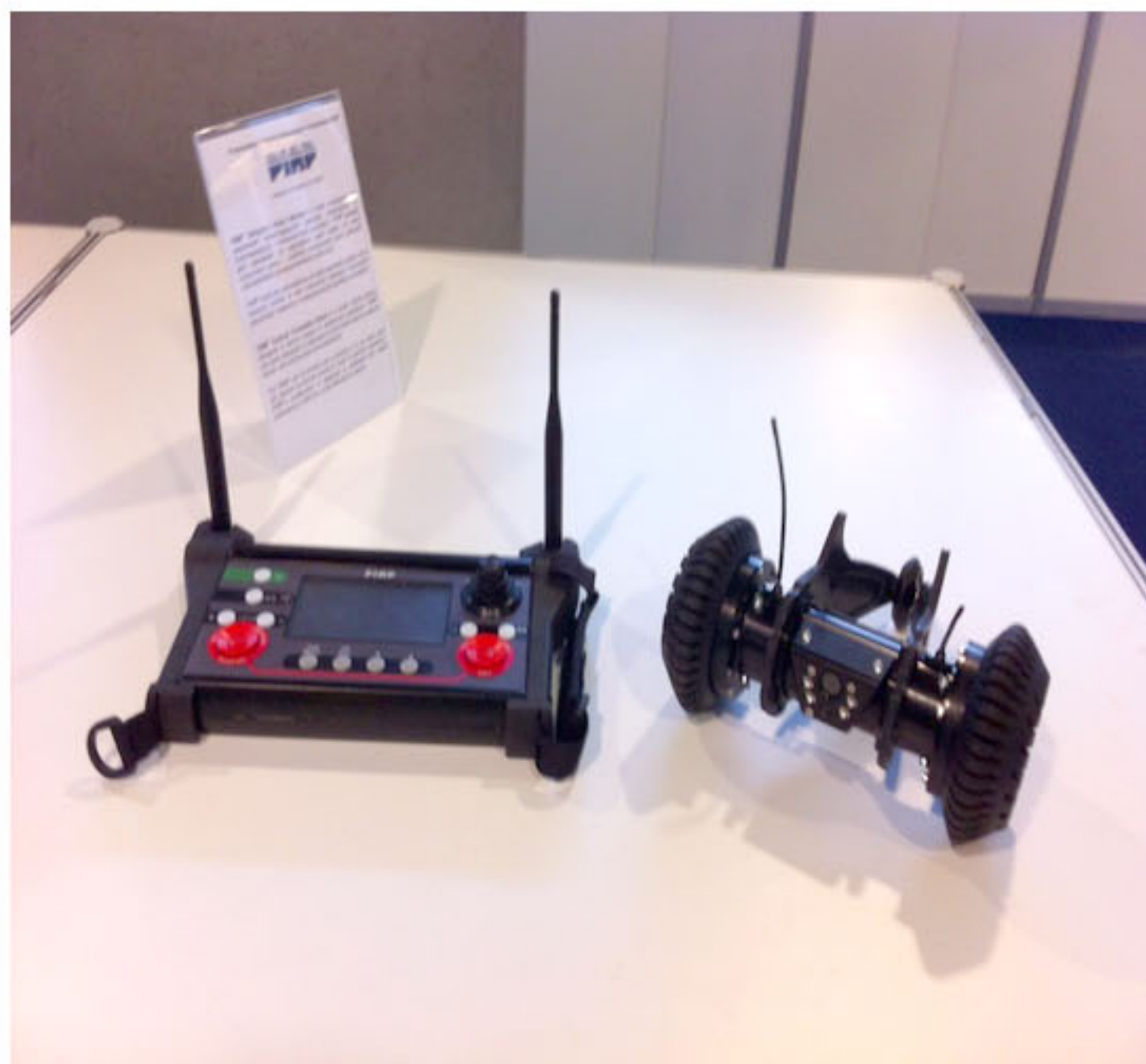
PIAP's award-winning next generation throw-bot, shown with its new control pad, which can operate three throw-bots and deploy flash-bang grenades.
