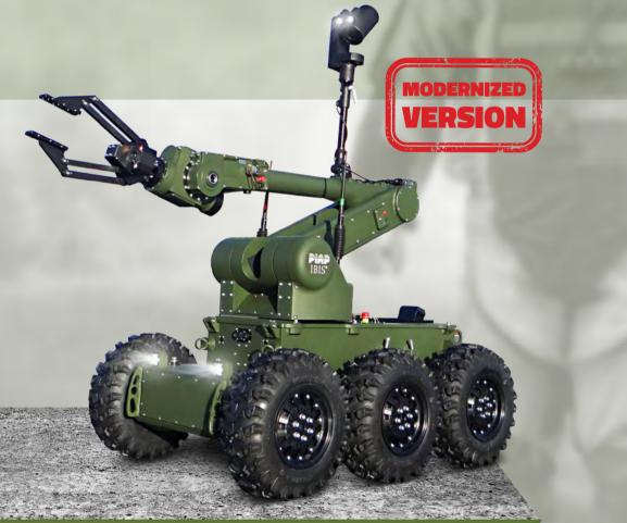
IBIS® is a fast robot (10 km/h). Special design of mobile base suspension ensures optimum wheel contact with the ground. Precision drive system ensures fluidity of the movement of every part of the robot, at any speed.
