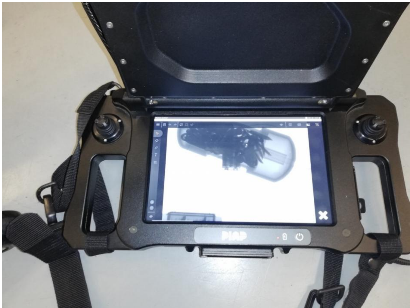
The remote console allows for scanning from a safe distance / Photos: PIAP
