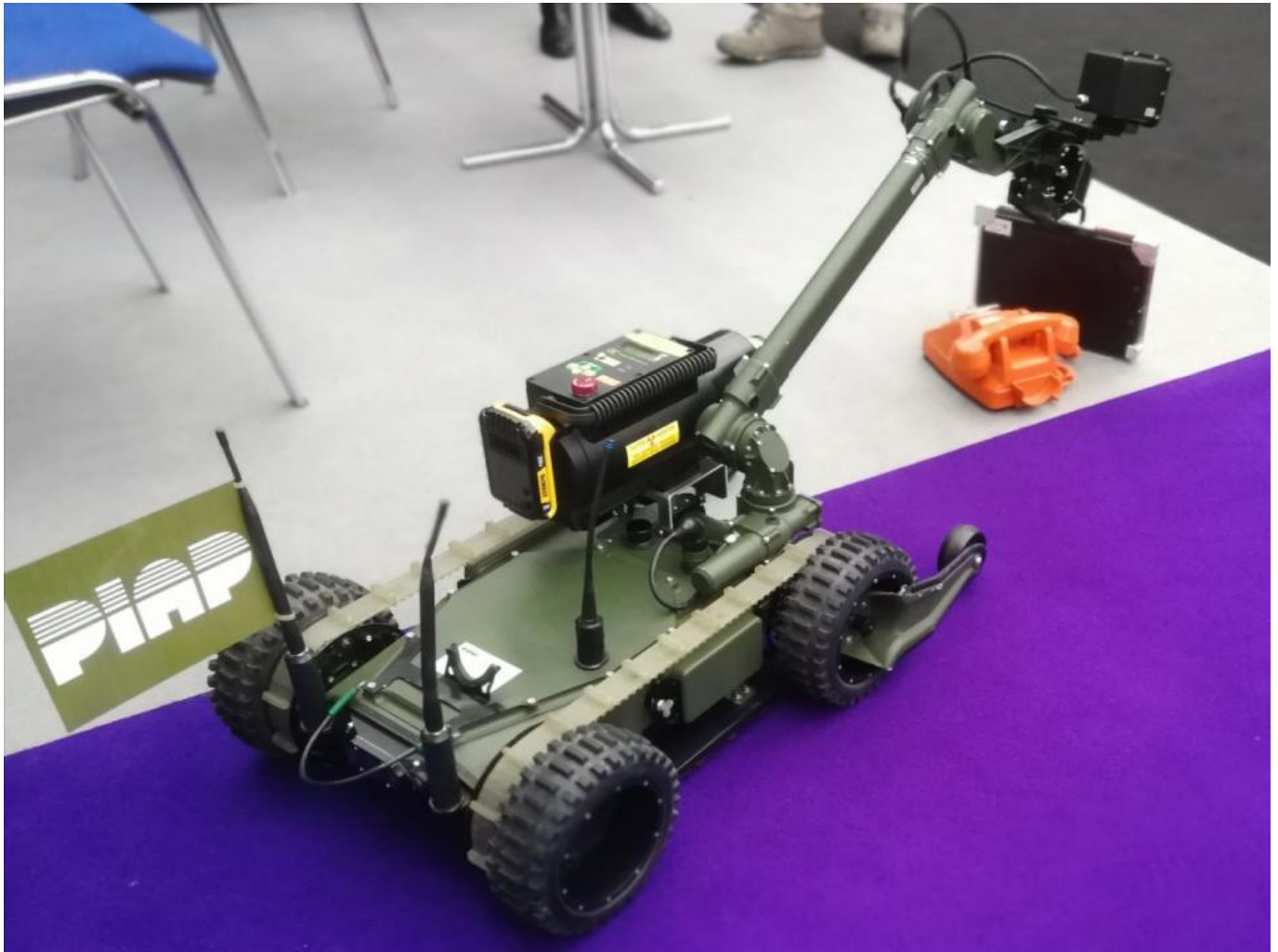
PIAP FENIX with an integrated PRÓTOS X-ray imaging system
