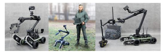
The PIAP GRYF bomb disposal robot is tailored to carry out hazardous materials neutralization tasks, explosive ordnance disposal included. The robot can be employed to safely identify, pick up, and transport suspicious objects, to the location where they could be safely neutralized. In extreme scenarios, the neutralization could take place in locations where the hazardous materials are discovered – in circumstances as such, the robot's accessories can be used.
